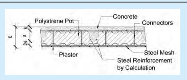
a = thickness of core; b = thickness of concrete; c = overall thickness
