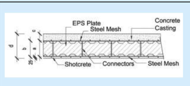
a = EPS Nominal Thickness (variable between 80 mm to 160 mm); b = Distance between thickness steel meshes (a + 10 mm);
