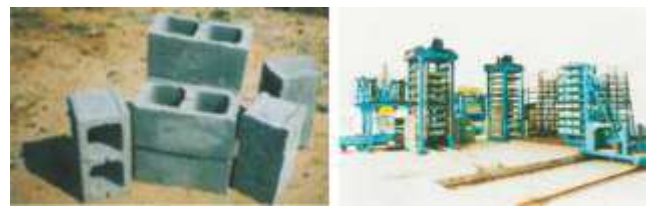
Figure 6 : Concrete Hollow Block and production machine
